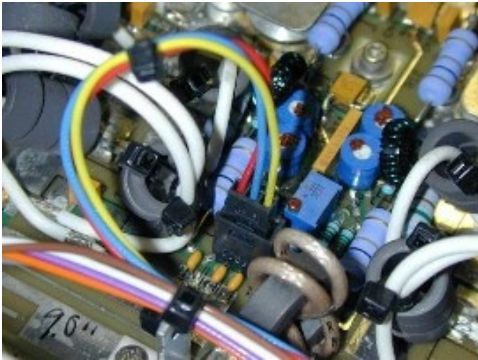
Gate bias/alarm connector & over temp
