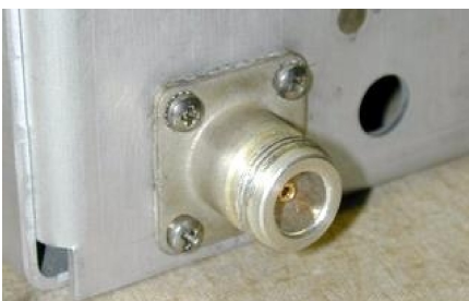
New RF output connector on chassis
