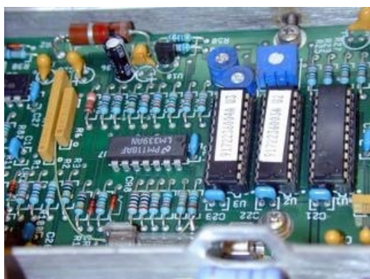
Control board, showing 3 PALs (center) and problem resistor R39 (upper left)
