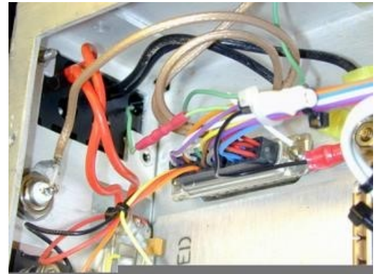
Internal wiring of Jones strip and new RF input connector
