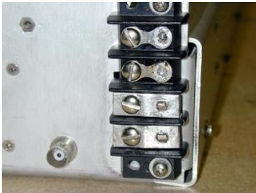
RF input connector & Cinch Jones terminal block modified for heavy DC input
