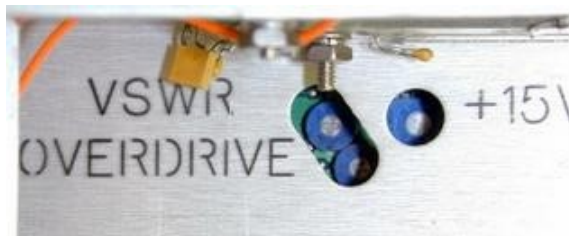
Control Board VSWR & Overdrive Adjustment Pots
