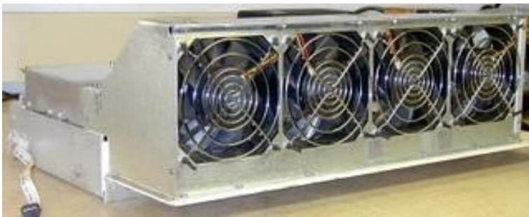
Completed Air Plenum
