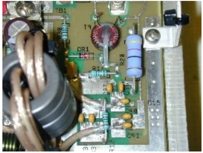
RF balance transformer and alarm
