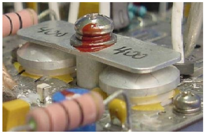
Device clamp to insure good thermal
